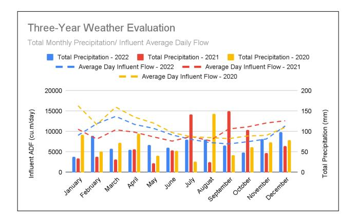
The facility operated at 60% of its Rated Capacity over the reporting period which is a marked improvement over the last three years. The Owner has spent several million dollars over the last six years to upgrade its WWTP and Wastewater Collection System (WWCS) infrastructure which is being realized in the Influent flows in an effort to extend the lifespan of the facility and reduce sources of I&I in the WWCS.
